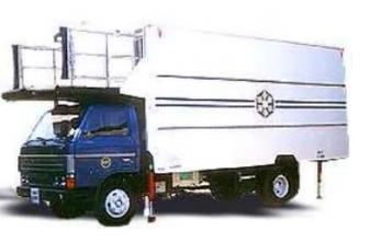
Height range:Standard cabin (2700 to 6000 mm),Half cabin (1600 to 600 mm).Chassis :16 tonne GVW.Payload :Ranging from 1500 kg to 4000 kg.
