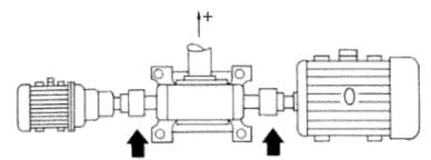
**OVERRUNNING**: Freewheel clutches are capable of overrunning at either the inner or outer race. This application is mainly required in stand by drives and compound drives Fig.2 shows a dual speed drive. Here two prime movers are connected to the input shaft of a gearbox through Freewheel clutch-couplings.
