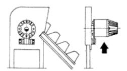
**BACKSTOPPING:** In Backstopping applications, Freewheel clutches are used to prevent reverse rotation of drive shafts. With the outer race of the clutch anchored to a stationary member, the inner race can overrun freely in one direction of rotation, reverse rotation is instantaneously prevented by the automatic engagement of the clutch. Fig. 3 shows a sprag clutch used as a Backstop on head shaft of a bucket elevator.
