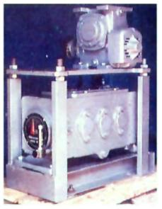
Britex Industries has come up with an innovative solution of variable drive variation at very low rpm. The system comprises of a basic P.I.V. unit with a worm hear stacked on top of systematic structure. The advantages of the system are as follows: Immediate delivers, compared to normal four months delivery scheduleIndividual components are detachable, and thereafter easily accessibly to maintenanceAnd replacements. Change of axis and shaft handing is also possible.
