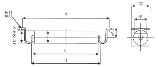
ROLLER BODY: The roller body is made of special ERW tube with close tolerance ensuring, smooth, shock-free and eccentricity free, running with minimum diameteral runout.
