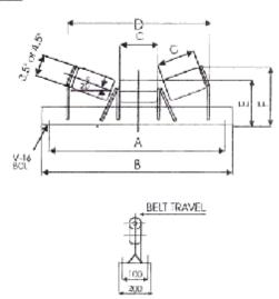
ROLLER BODY: The roller body is made of special ERW tube with close tolerance ensuring, smooth, shock-free and eccentricity free, running with minimum diameteral runout.
