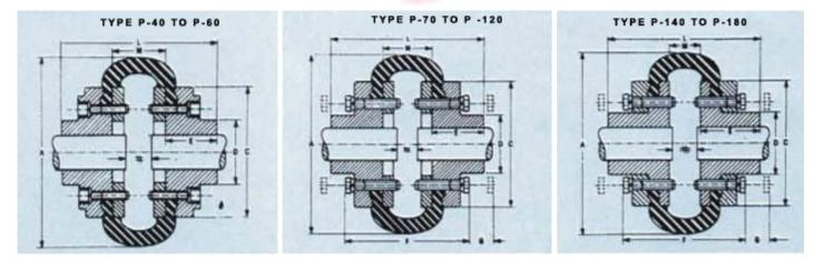
Tyre Couplings with a choice of 3 types of tyres and a range of 14 sizes from 24 to
